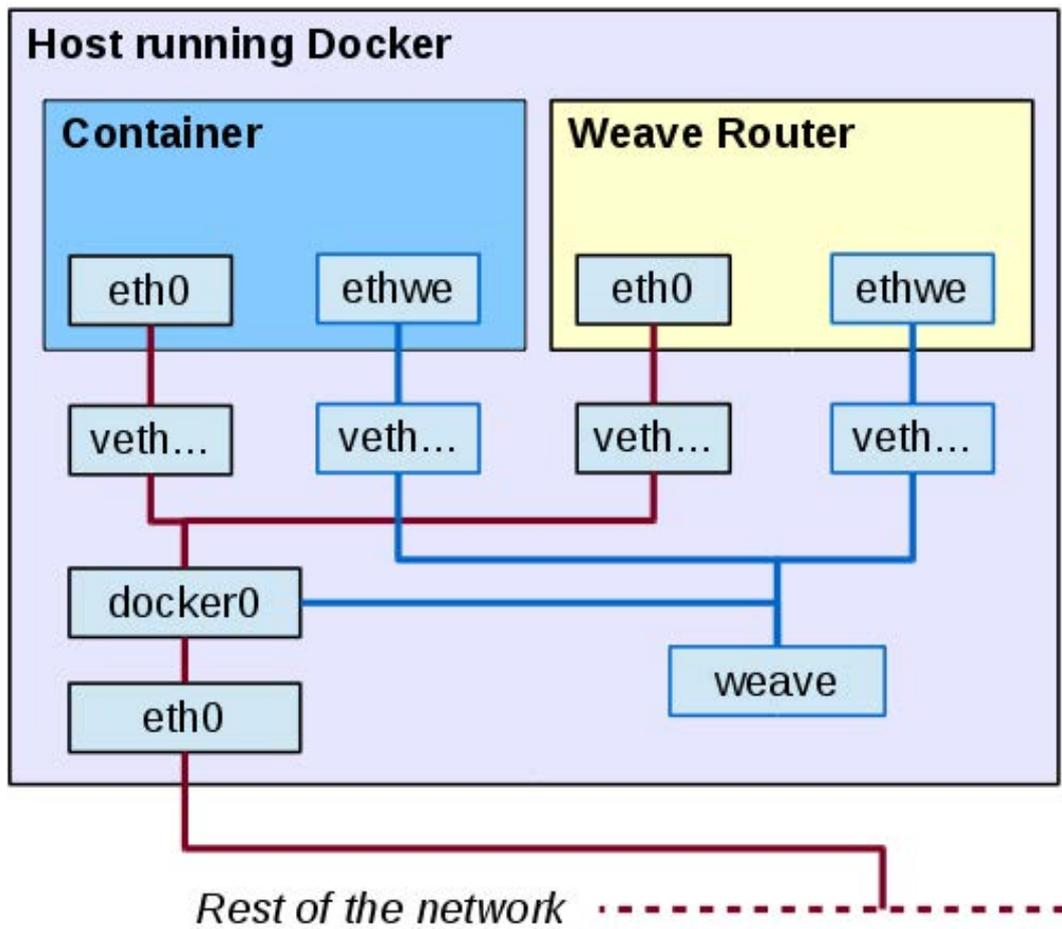
Figure 3. Weave adds several virtual devices to redirect some of the traffic eventually to other servers.
