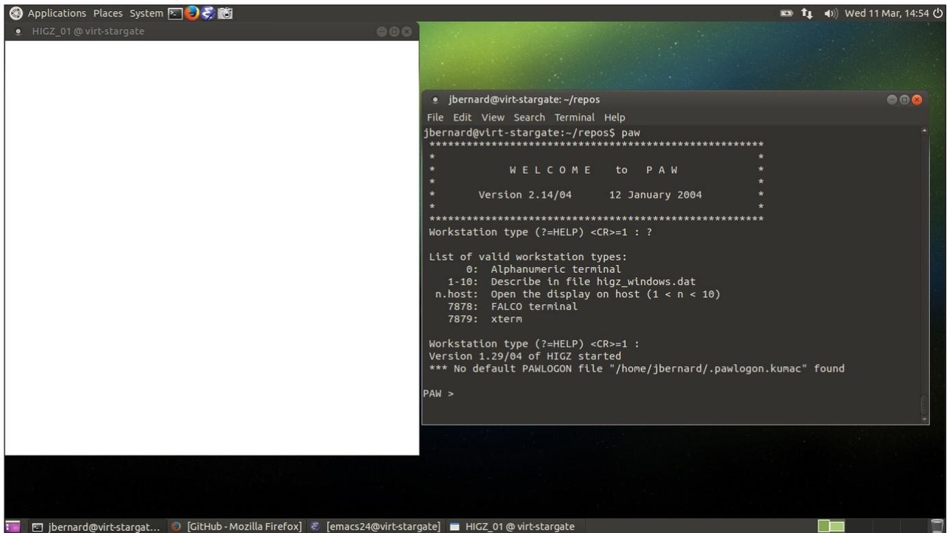
Figure 2. The default is to open a graphics window to draw your plots into, along with a command interface.
