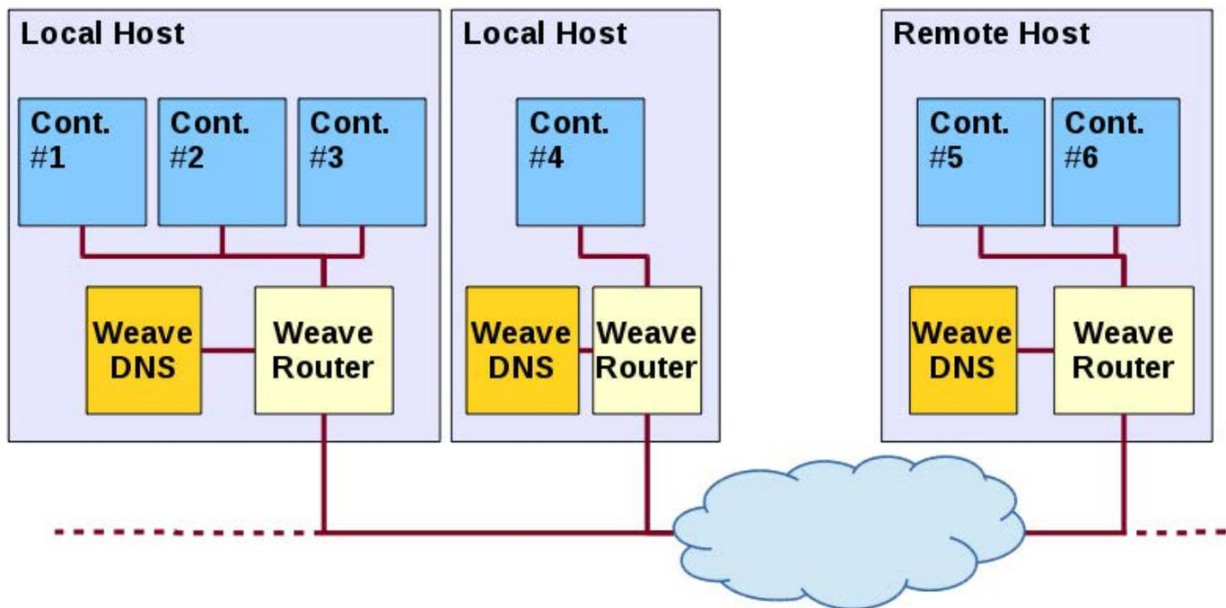
Figure 4. Using Weave, containers in local and remote networks connect to each other transparently; access is simplified with Weave DNS.
