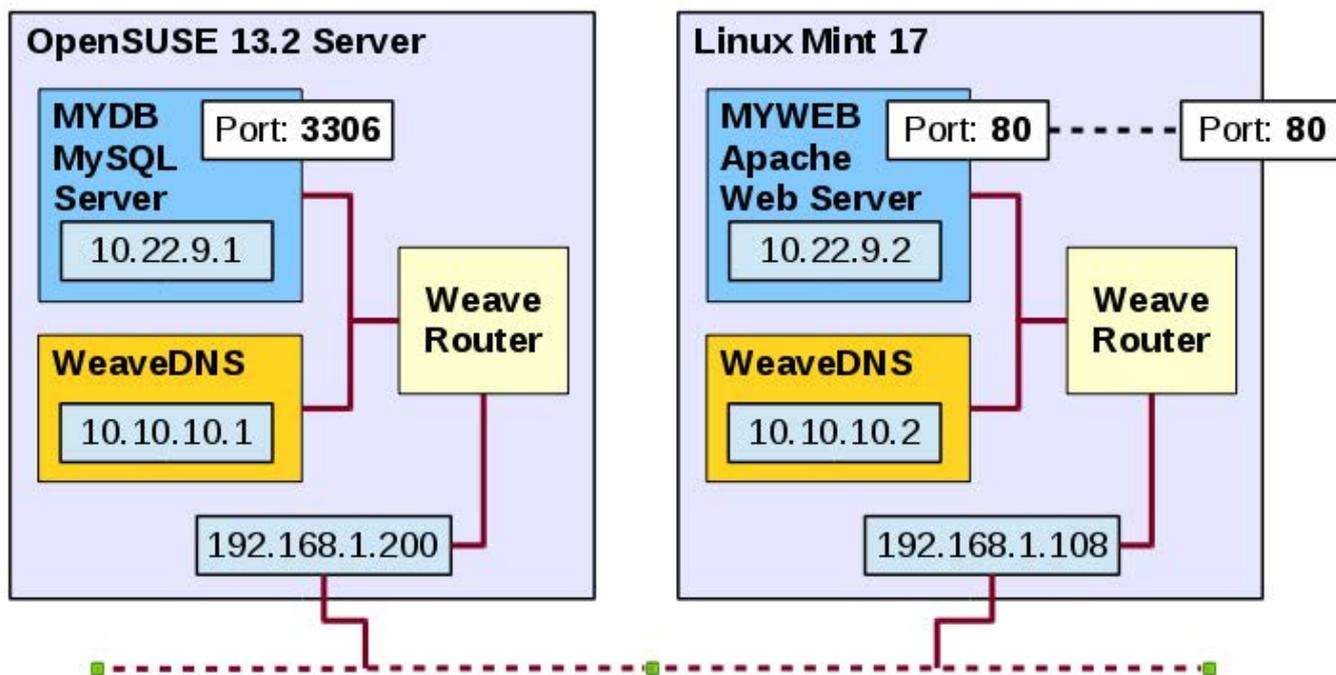
Figure 5. The final Docker container-based system, running on separate systems, connected by Weave.
